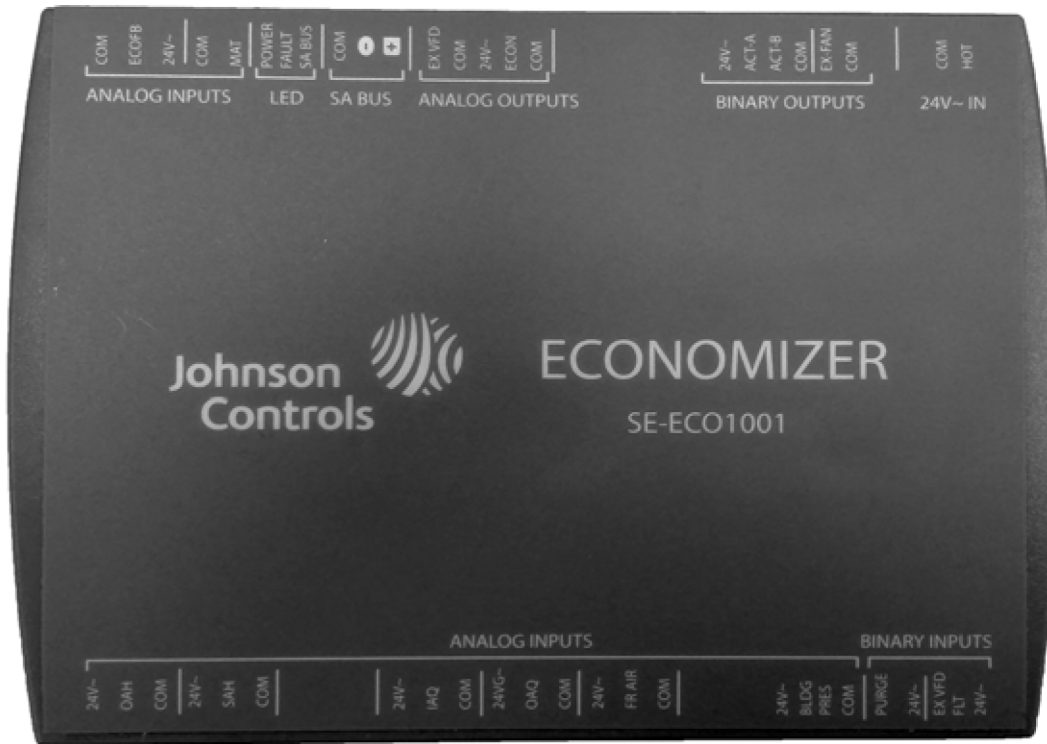
Figure 26: SE-ECO1001-1 economizer controller
