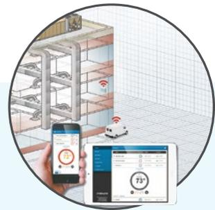
An optional Mobile Access Portal (MAP) gateway with Wi-Fi® hotspot provides access to commissioning, configuration and maintenance logs using a mobile smart device for **fewer trips to the job site or the roof to diagnose issues.**
